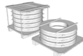
Two or more coils on a pallet, axis vertical wooden battens between
